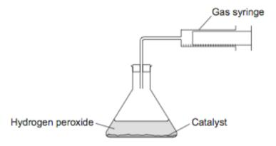
A powdered catalyst is added to the hydrogen peroxide.
