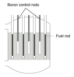
The fuel rods are made of a radioactive element. The boron control rods are used to control the reaction inside the reactor. Boron atoms absorb neutrons safely.
