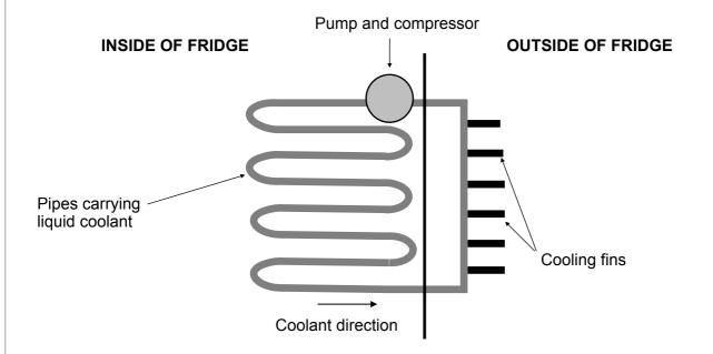
The cooling mechanism works in the following way:
